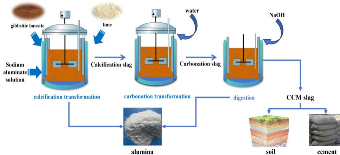
Figure 2. Process flow for the preparation of cement from the transformation products of bauxite or red mud treated by the calcic carbonation method.
